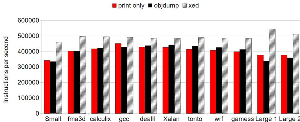
Figure 4.10: Performances of the MADRAS disassembler on Intel 64 files, compared with **objdump** and **XED**. The MADRAS disassembler directly prints instructions without allocating structures (*print only* mode).
