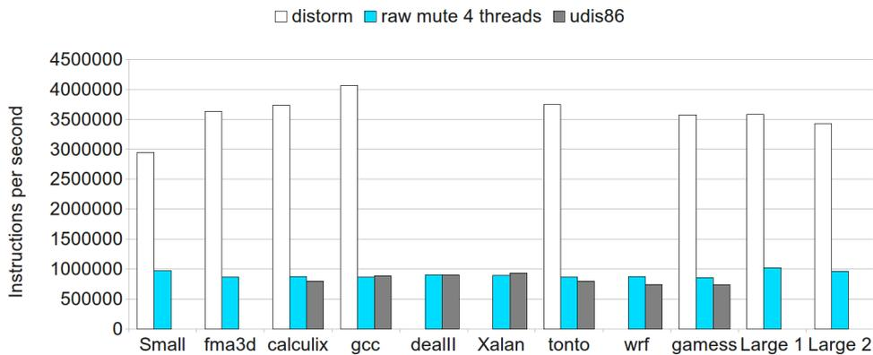
Figure 4.17: Performances of the MADRAS disassembler in 4 threaded mode on Intel 64 files, compared with `udis86` and `distorm`. For this test, the *raw mute* mode was used for MADRAS.
