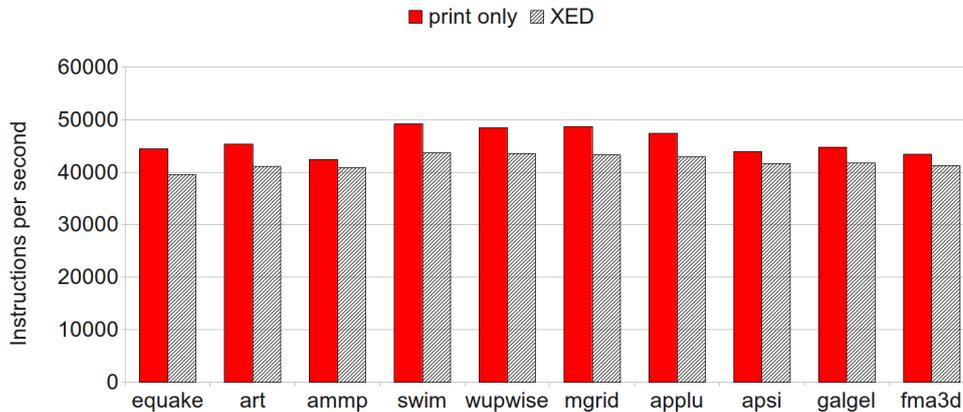
Figure 4.12: Performances of the MADRAS disassembler on Xeon Phi coprocessor files, compared with **XED**. The MADRAS disassembler directly prints instructions without allocating structures (*print only* mode). Unlike the others, those tests were performed on a Xeon Phi system, causing a lower speed for both tools.
