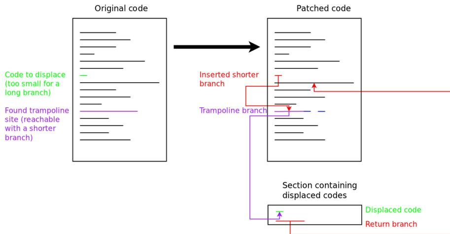
Figure 5.3: Illustration of the principle of using trampolines to displace code
