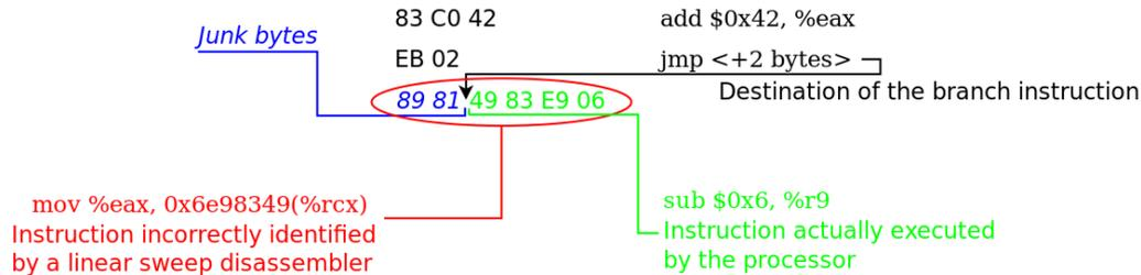
Figure 4.2: Example of an obfuscated Intel 64 code. If the disassembler misses the `jmp` instruction used to skip the junk bytes, it will process them and the following instruction as a single instruction very different from the actual one.
