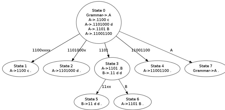
Figure 3.1: First iteration of the FSA generated from the sample grammar.
