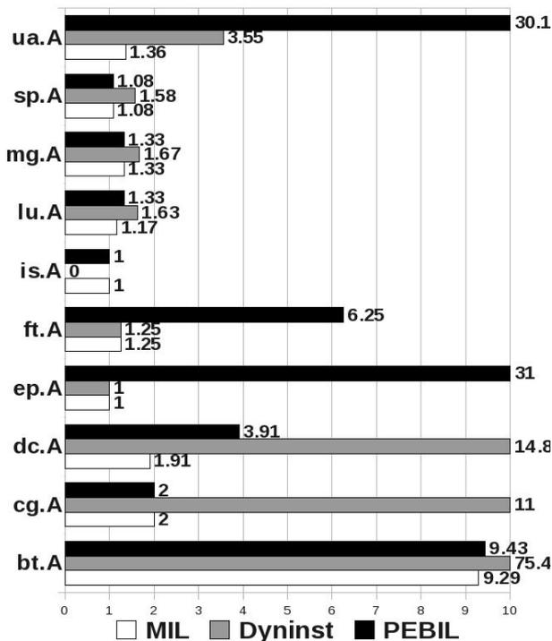
Figure 5.5: Comparing overhead time on NAS OMP benchmarks for MIL, Dyninst and PEBIL using TAU. X axis reports the overhead ratio compared to the original run. Lower is better. Overhead ratios greater than 10 are cut. A zero ratio means a crash at runtime. Source: [43]
