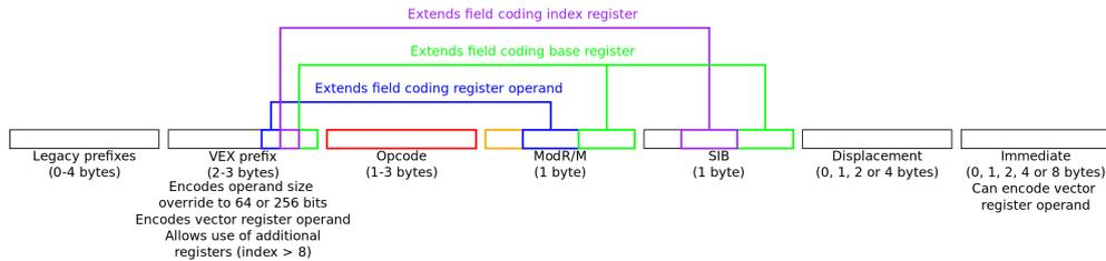
Figure 2.3: Overview of the structure of an encoded AVX Intel 64 instruction, focussing on the use of the VEX prefix.
