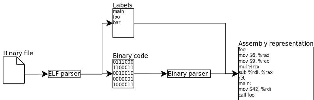
Figure 4.7: Description of the handling of binary files by the MADRAS disassembler.
