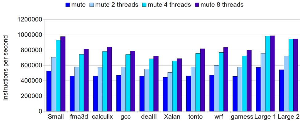
Figure 4.15: Performances of the MADRAS disassembler on Intel 64 files, for various number of threads. For this test, the *mute* mode was used for MADRAS.
