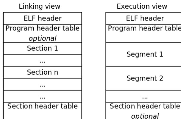
Figure 2.4: Representation of the structure of an ELF file, distinguishing between relocatable and executable files. Source: [14].
