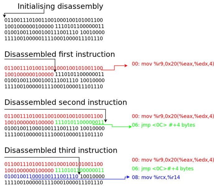
Figure 4.5: Example of a linear sweep disassembly on Intel 64 code.
