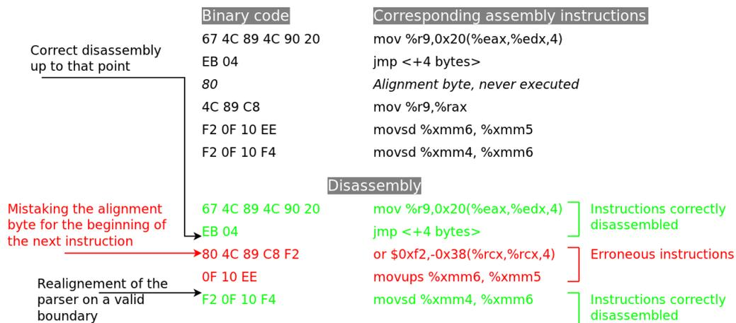
Figure 4.1: Example of a disassembly being thrown off course and returning erroneous instructions. The code used is Intel 64 with instructions of different binary length.
