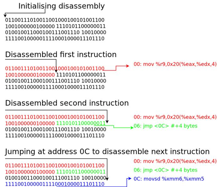
Figure 4.6: Example of a recursive traversal disassembly on Intel 64 code.
