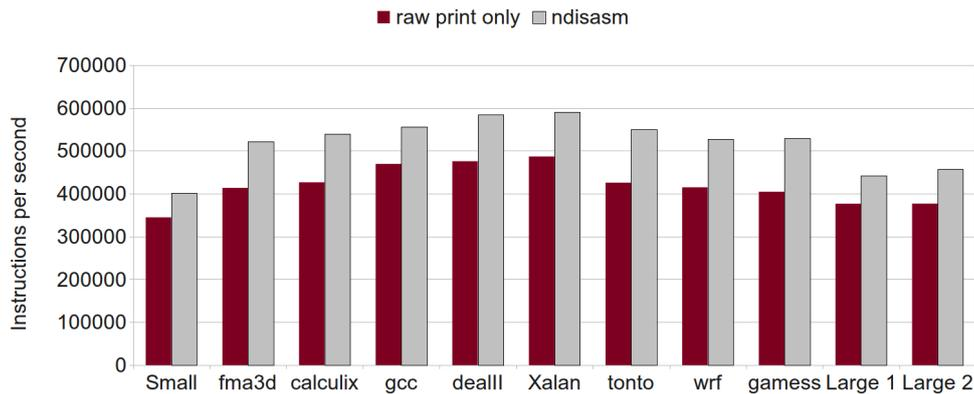
Figure 4.13: Performances of the MADRAS disassembler on Intel 64 files, compared with **ndisasm**. The MADRAS disassembler directly prints instructions without allocating structures and does not parse the ELF file (*raw print only* mode).
