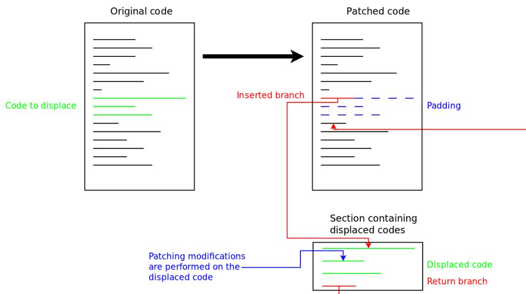
Figure 5.2: Patching a file using code displacement
