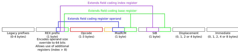
Figure 2.2: Overview of the structure of an encoded Intel 64 instruction, focussing on the use of the REX prefix.
