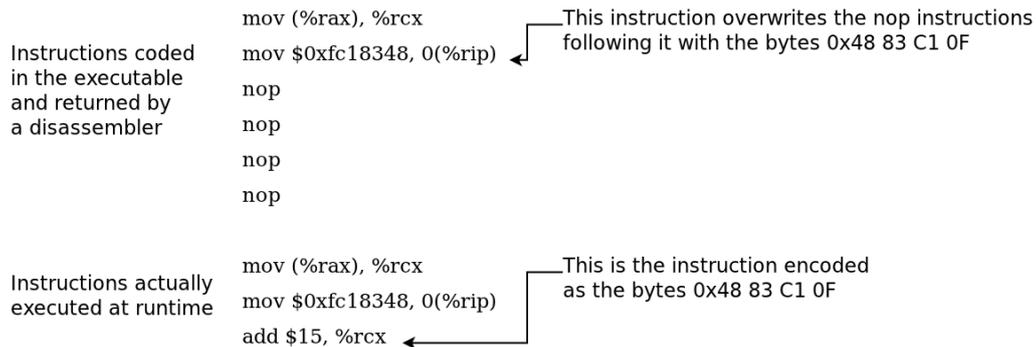
Figure 4.3: Example of a simple self rewriting Intel 64 code for a single instruction.
