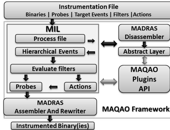
Figure 5.4: MIL: MAQAO Instrumentation Language and its integration in the MAQAO framework. Source: [43]
