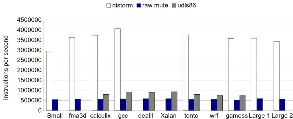
Figure 4.14: Performances of the MADRAS disassembler on Intel 64 files, compared with **udis86** and **distorm**. The MADRAS disassembler allocates structures representing instructions without printing them and does not parse the ELF file (*raw mute* mode). Missing values indicate that the tool crashed for all tests on this file.
