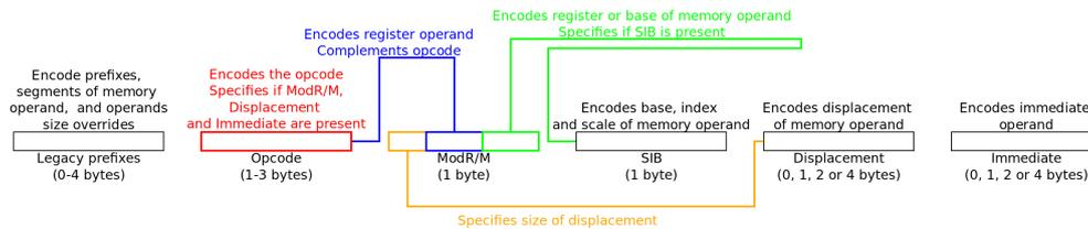
Figure 2.1: Overview of the structure of an encoded IA-32 instruction, describing the relationships between the various bytes involved in the encoding.
