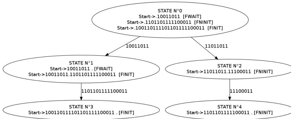
Figure 3.4: Part of an automaton handling instructions FWAIT, FNINIT and the macro instruction FINIT. State 1 is a shift/reduce state; if the transition over value 1101101111100011, which would lead to the reduction of symbol 100110111101101111100011 corresponding to macro instruction FINIT, fails, symbol 10011011 (FWAIT) is reduced instead.
