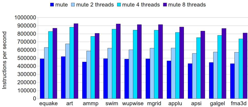
Figure 4.16: Performances of the MADRAS disassembler on Xeon Phi coprocessor files, for various number of threads. For this test, the *mute* mode was used for MADRAS.
