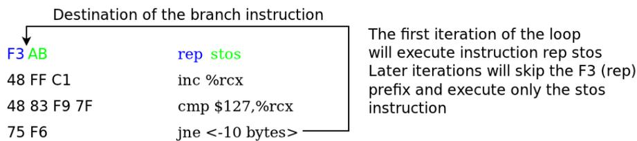
Figure 4.4: Example of the use of overlapping instructions in Intel 64 code involving the `stos` and `rep stos` whose opcodes differ only by a prefix.
