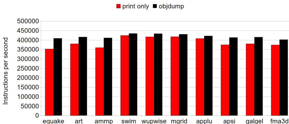
Figure 4.11: Performances of the MADRAS disassembler on Xeon Phi coprocessor files, compared with **objdump**. The MADRAS disassembler directly prints instructions without allocating structures (*print only* mode).
