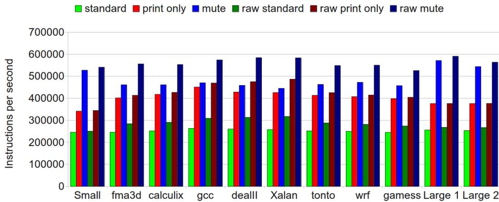
Figure 4.8: Performances of the MADRAS disassembler on Intel 64 files, for various operating modes. In *print only*, the instructions are printed directly without allocating structures, while for *mute*, the structures are allocated and destroyed but nothing is printed. Finally, in *standard*, the structures are allocated, printed and freed. *Raw* modes skip the parsing of the ELF file.
