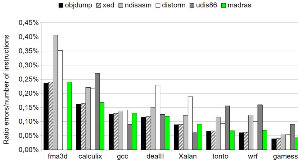
Figure 4.18: Comparison of error ratios between other disassemblers and MADRAS for Intel 64 executables. In this test lower values represent a better accuracy.
